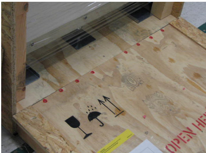
Figure 2-7 Cabinet ramp and crate base
