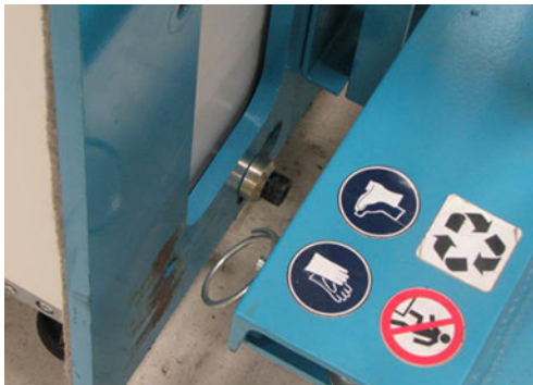
Figure 2-11 Mounting lugs and dolly keyhole slots
