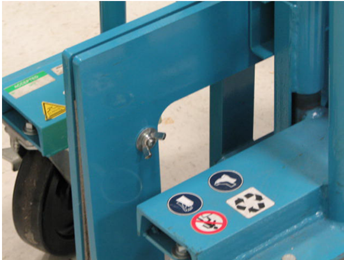
Figure 2-10 Separating the two dolly halves
