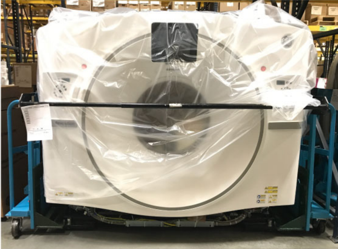
Figure 14-1 Gantry with Shipping Dollies and Side Rails
