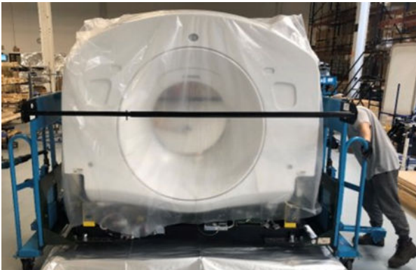
Figure 14-2 Gantry with old Shipping Dollies and Side Rails
