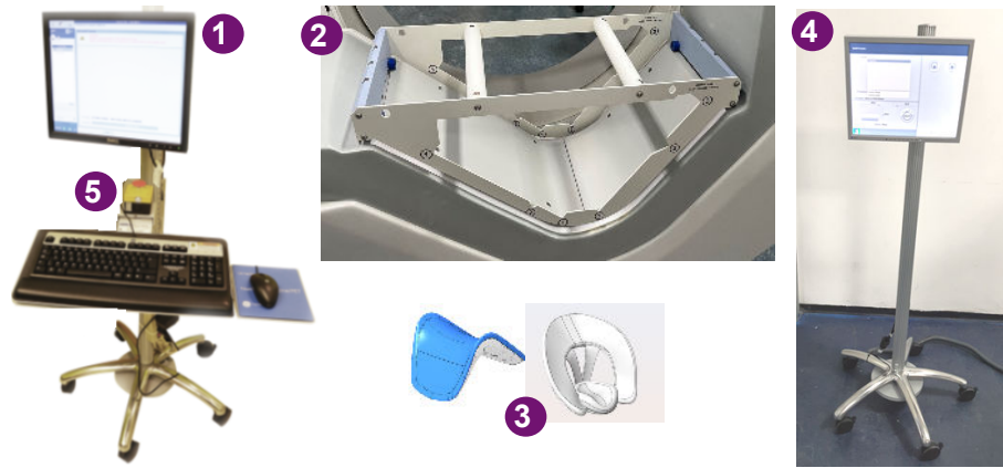
Figure 2-2 Scan Room Moving Components
