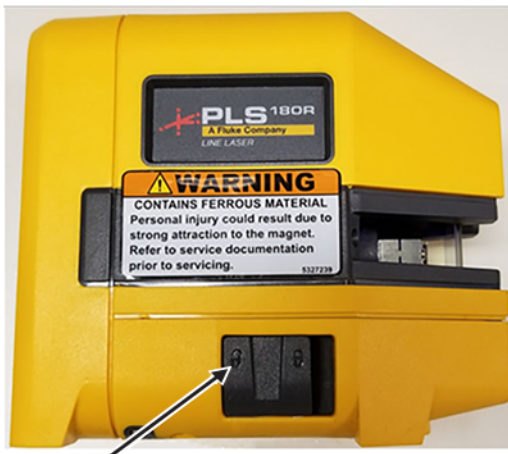
Figure 5-12 Laser level in self-leveling mode (unlocked position)
