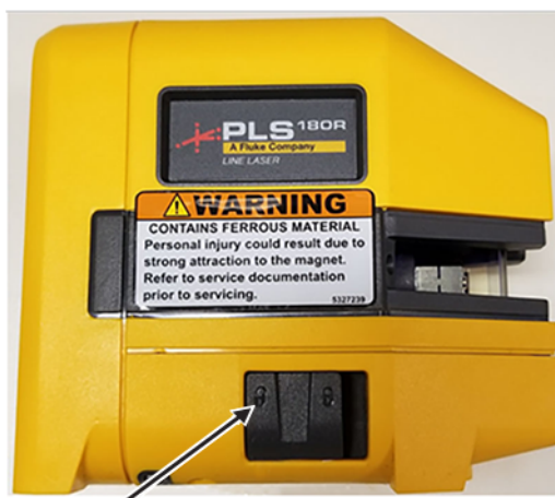
Figure 6-12 Laser level in self-leveling mode (unlocked position)
