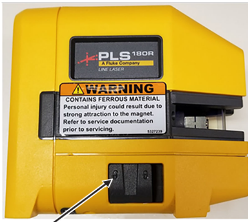
Figure 5-9 Laser level in self-leveling mode (unlocked position)
