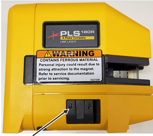
Figure 6-6 Laser level in self-leveling mode (unlocked position)
