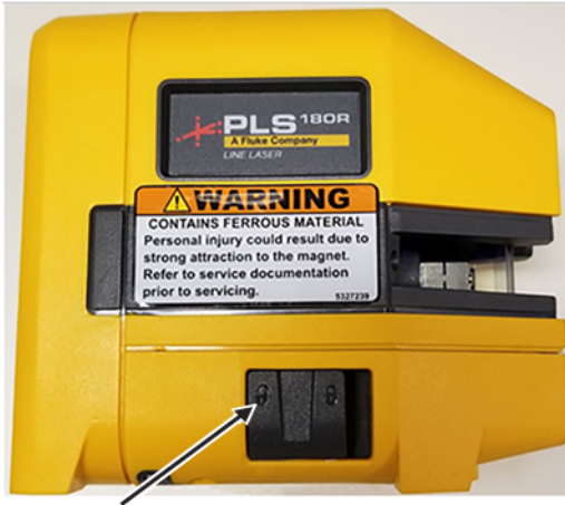
Figure 7-11 Laser level in self-leveling mode (unlocked position)
