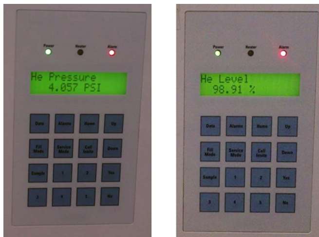
Figure 3-9 Magnet Monitor front panel user interface, He Pressure (psig) (left) and He Level (%) (right)
