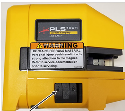
Figure 6-6 Laser level in self-leveling mode (unlocked position)
