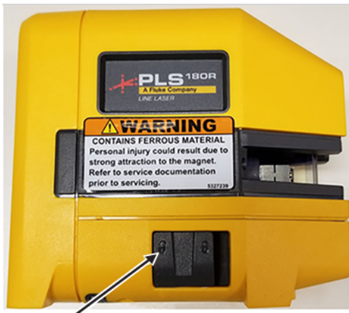
Figure 5-10 Laser level in self-leveling mode (unlocked position)
