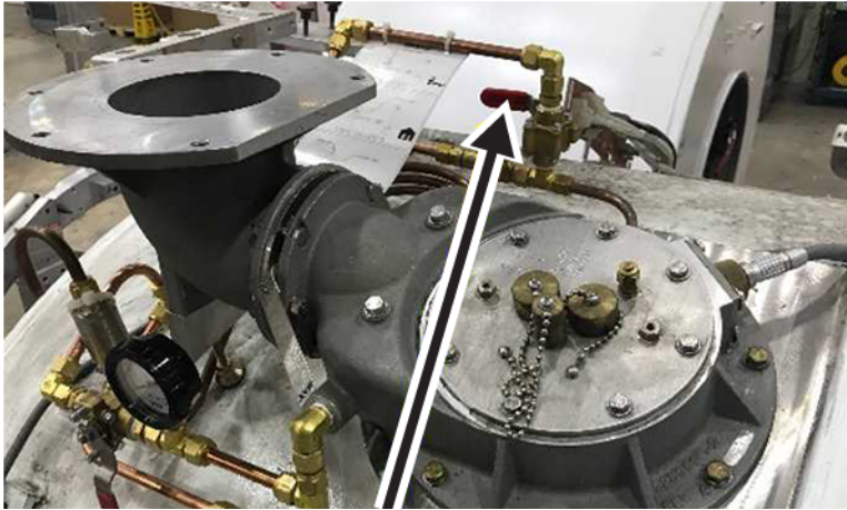
Figure 3-12 V3 valve in the closed position
