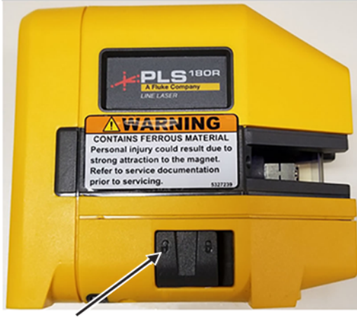
Figure 6-12 Laser level in self-leveling mode (unlocked position)
