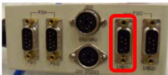
Figure 3-9 Typical instrumentation connector assembly ports
