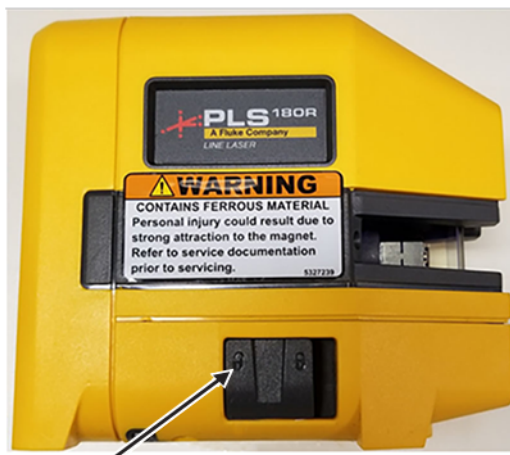
Figure 5-7 Laser level in self-leveling mode (unlocked position)
