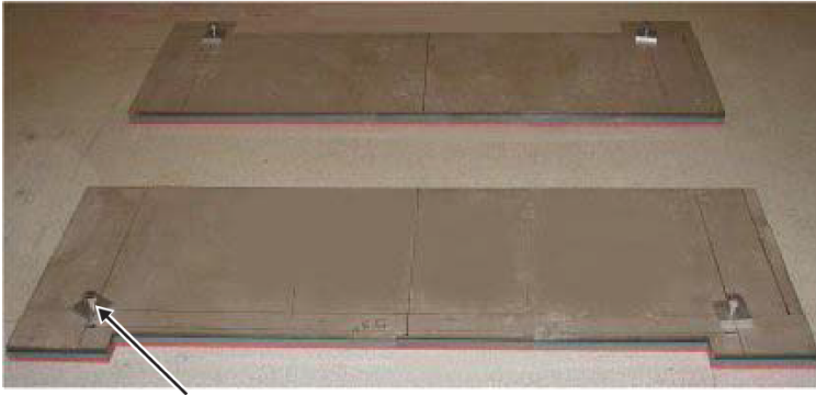
Figure 7-1 Surface mounted non-SV vibroacoustic damping mats
