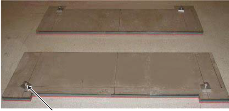
Figure 6-1 Surface mounted non-SV vibroacoustic damping mats
