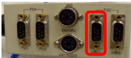
Figure 3-6 Typical instrumentation connector assembly ports
