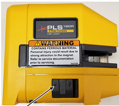
Figure 6-12 Laser level in self-leveling mode (unlocked position)
