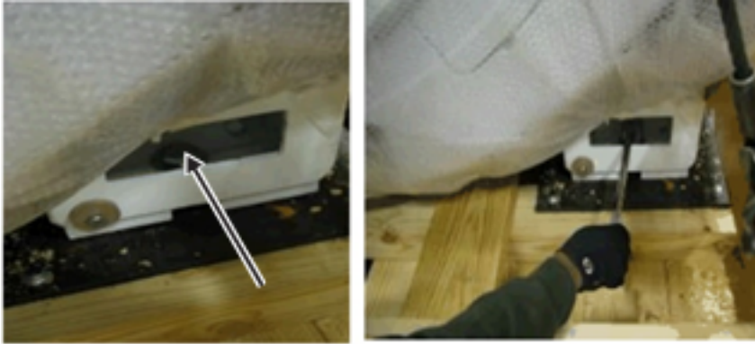
Figure 2-8 Unbolting the magnet from a shipping pallet
