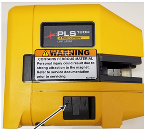
Figure 5-14 Laser level in self-leveling mode (unlocked position)
