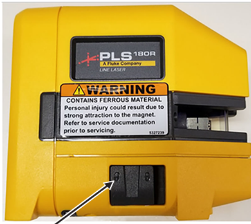
Figure 5-11 Laser level in self-leveling mode (unlocked position)
