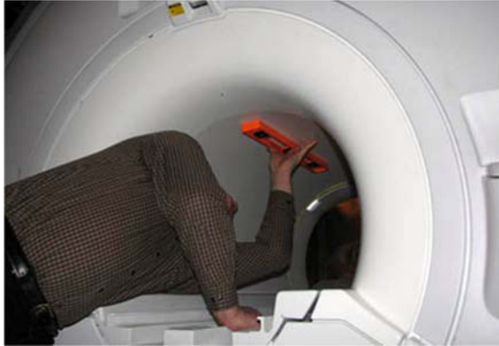
Figure 6-12 Magnet leveling, front-to-back
