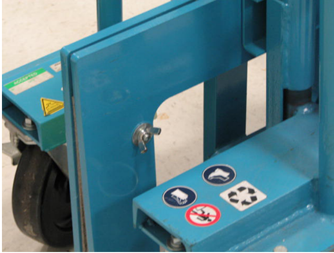
Figure 3-12 Separating the two dolly halves
