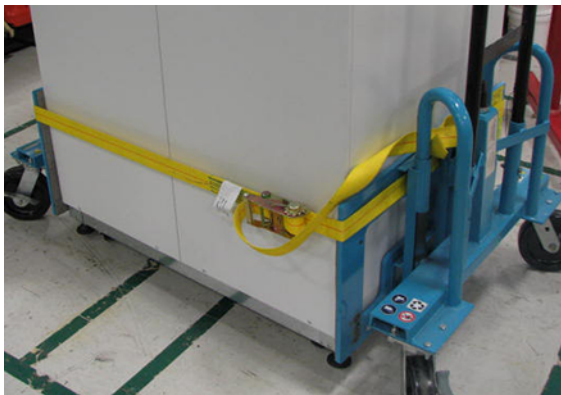
Figure 3-15 Securing the cabinet on the dolly
