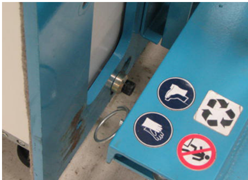
Figure 3-13 Mounting lugs and dolly keyhole slots
