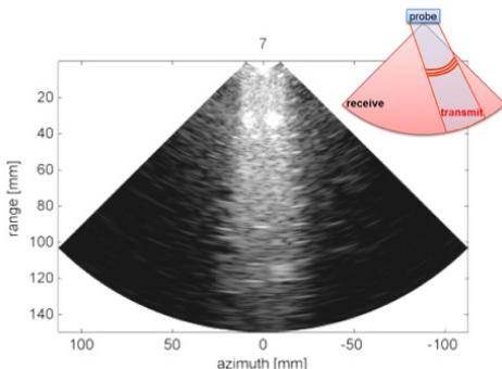
Figure 1. Plane wave imaging, schematic illustration and tissue phantom recording.
